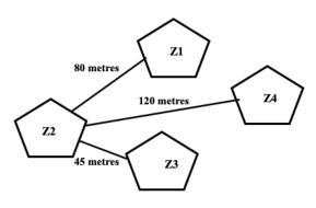
iii. **Repeater:** To be placed between Block Z2 to Z4 as distance between them is more than 100 metres.
